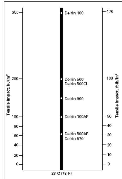
Figure 2 Delrin Izod impact properties
