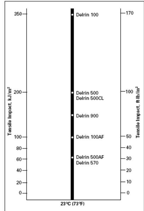
Figure 2 Delrin Izod impact properties
