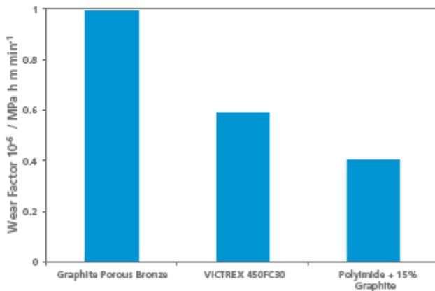
Figure 30: Lpv for a Range of Bearing Materials at 20°C (68°F), with v = 3 m s<sup>-1</sup> (600 ft min<sup>-1</sup>)
