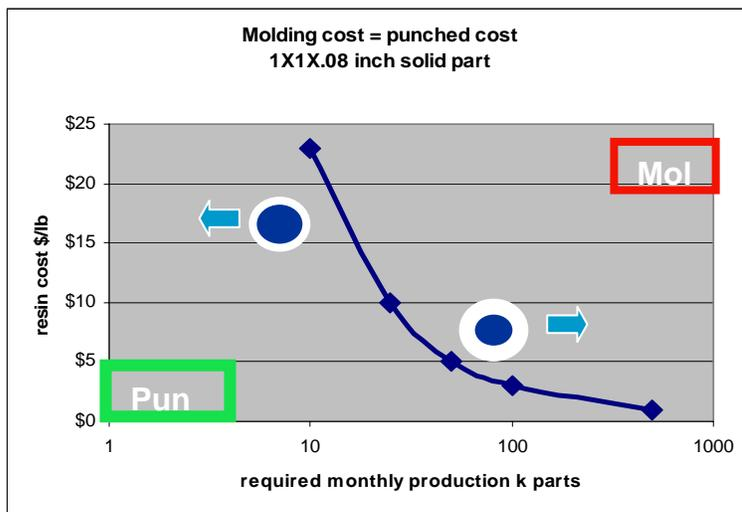
**Punching also requires the part to be flat from a geometric standpoint. Shoulder washers or beveled holes and edges would require subsequent machining. Parts of this nature are simply not competitive from a punching perspective. While there is some leeway depending on the material, in general punching requires the parts OD minus its ID to be greater than twice the thickness.**
