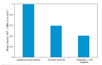
Figure 30: Lpv for a Range of Bearing Materials at 20°C (68°F), with  $v = 3 \text{ m s}^{-1}$  (600 ft min<sup>-1</sup>)
